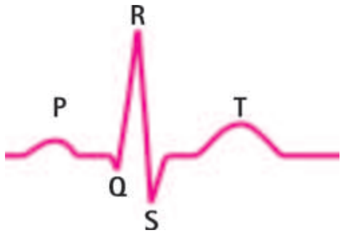
Figure 14: Typical second lead ECG signal. P, Q, R, S, T denotes distinct phases of the ECG recording.
