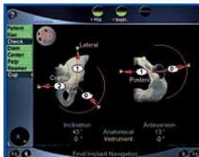
Screen image of the planned orientation for cutting out the socket bed and implanting the artificial socket.
