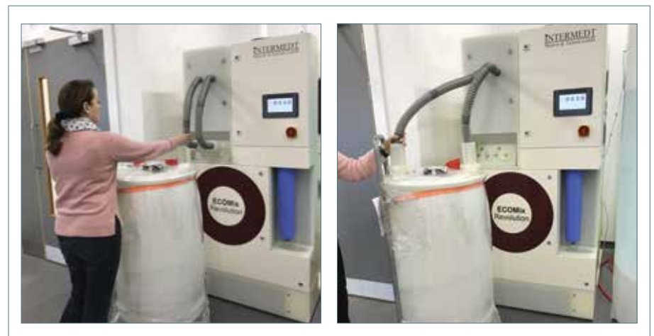
Figure 3: The EcoCart powder cartridge is supplied in a sealed drum placed on an integrated trolley for safe and easy movement. Connecting the EcoCart to the EcoMix device is extremely straightforward with built-in controls to avoid input errors. Empty EcoCart containers are reusable.
