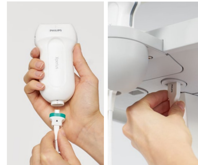
FIGURE 2 | Easy and quick attachable USB port connection at the transducer and at the Xperius Cart System.
