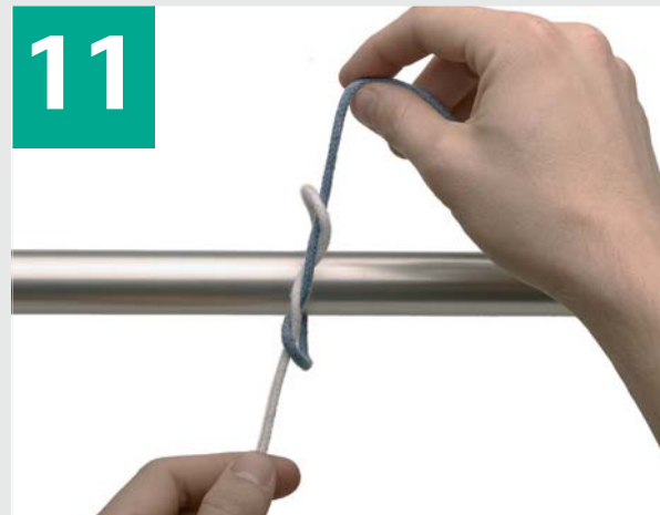
Tighten the knot by pulling blue thread away from you and white thread towards you.
