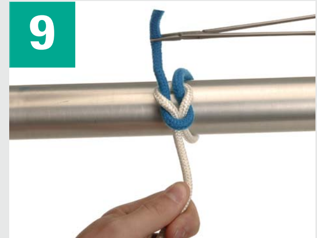
Pull blue strand away and white strand towards operator. A square knot should be obtained.
