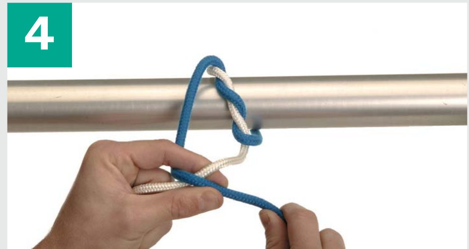
4 Hold blue strand between left index finger and thumb.
