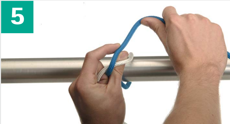
5 Place blue strand over white strand and hold it between left index finger and left thumb.
